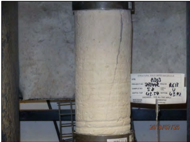
Front view (post-test)
